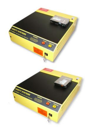
Rotate hard drive over magnetic field
